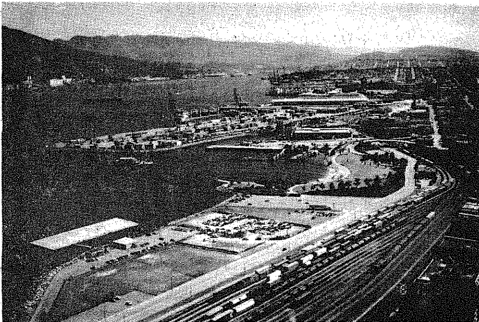
Figure 5.2.8 Intermodal operations among sea vessels, railroads, and motor carriers in Vancouver, B.C. harbor. (Photo by P. D. Prevedourous.)
